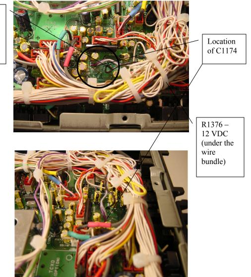
12 VDC can be taken from any point where it is convenient and the ground can be connected to any convenient point which is connected to the chassis ground. There are a number of suitable locations to connect 12 VDC and GND. We chose to connect to R1376 to get 12 VDC and to scrape clean a point near C1360 to tack to the board ground plane.
