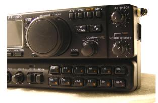
SGC mounted the switches on the FT900 on the right side when looking at the front panel.
