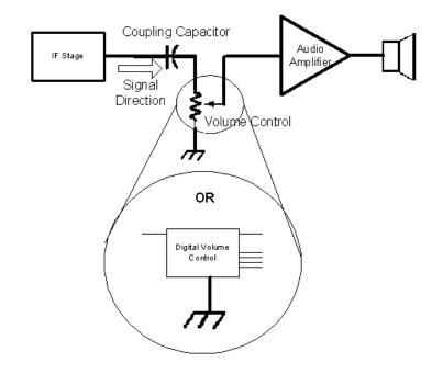
SGC recommends removing the C1174 coupling capacitor and connecting the audio in/audio out connections across where the capacitor was.
